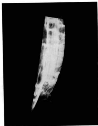
Fig. 13. Photograph of beam diffracted from a doubly-bent LiF monochromator.
